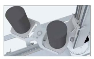
The "TwinFork" double gripper significantly reduces chip-to-chip time when changing pallets. This is an important factor for long transfer distances and short machining times.
